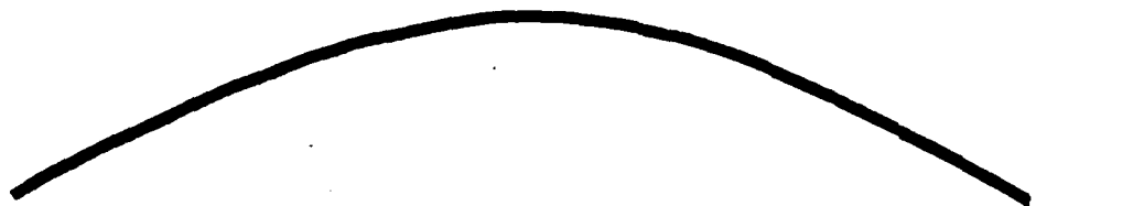
FIGURE 8. THE SHAPE WHICH THE STORE ATTEMPTS TO TAKE WHEN EXPOSED TO THE CORRESPONDING LOADINGS OF FIGURE 7
