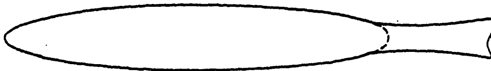
Prolate Spheroid of Fineness Ratio 6
