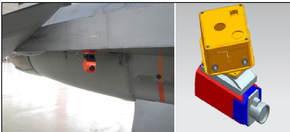
Figure 4-38: Rear Camera Adaptor and its Application Under the Fuselage of F-16.
