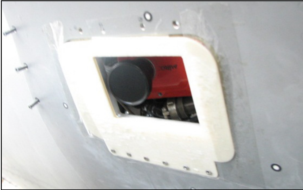
Figure 4-39: Camera Application Inside the Fuselage of F-16.
