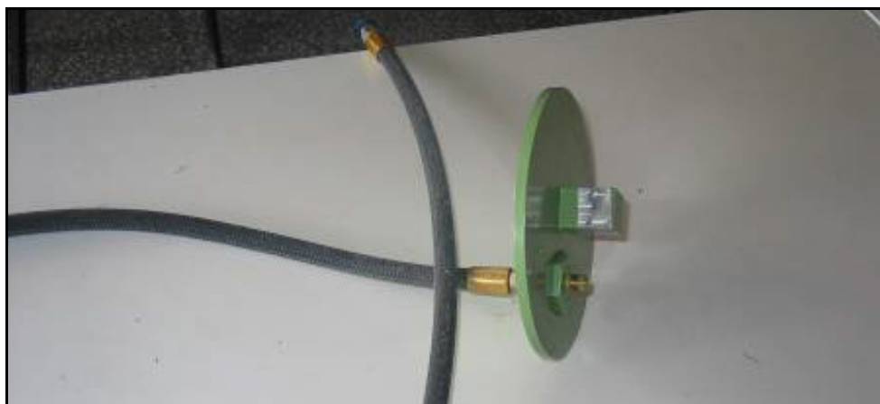
Figure 4-42: A Mechanical Interface for the Accelerometer Used in F-16 External Fuel Tanks.
