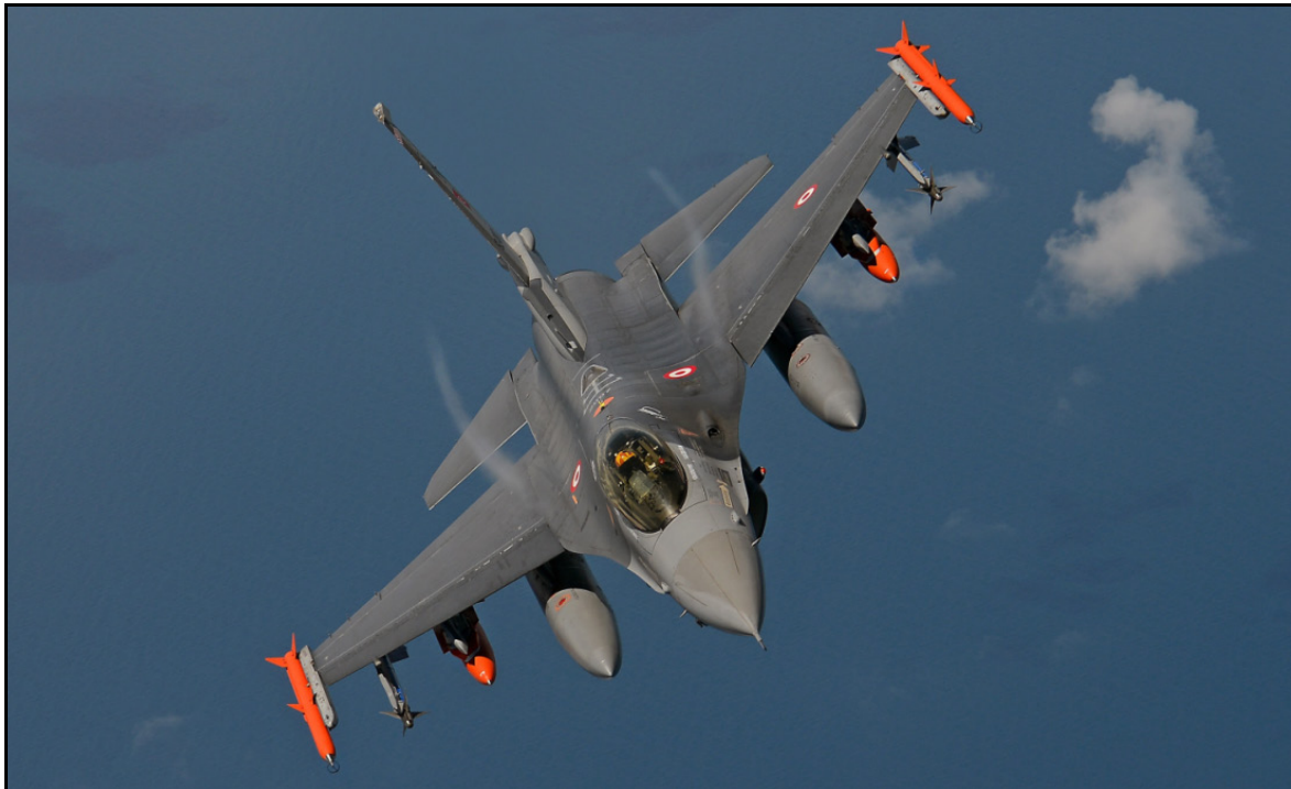
Figure 4-46: Flight Flutter Test on F-16 A/C for Newly Developed Munitions.
