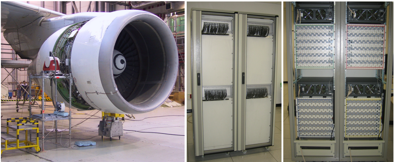
Figure 5. (Left) Engine shaker excitation. (Right) 700-channel LMS data acquisition system.
