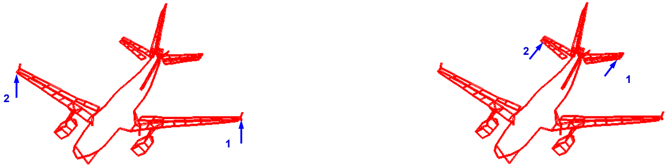
Figure 10. Shaker locations during vertical wing testing and longitudinal horizontal tail plane testing.
