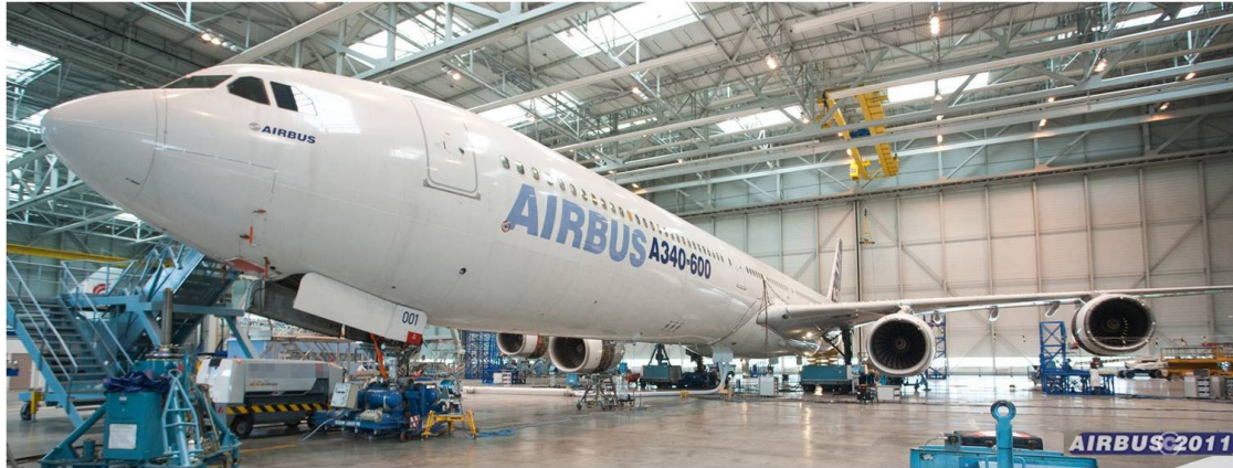
Figure 1 A340/600 aircraft during the GVT
