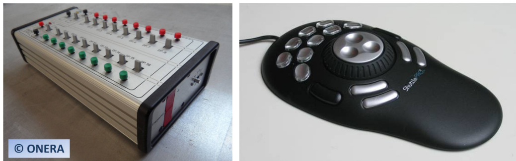
Figure 5 Excitation Force Control devices used by ONERA and by DLR
