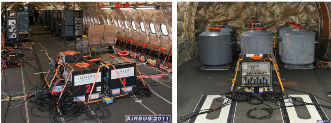
Figure 6 ONERA and DLR racks with LMS Scadas III inside the fuselage, linked with optical fibers
