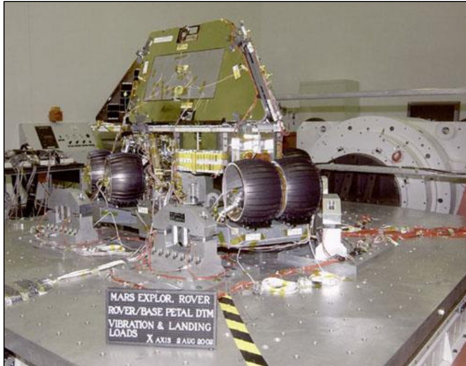
Figure 2—MER DTM Rover in Lateral Vibration Test
