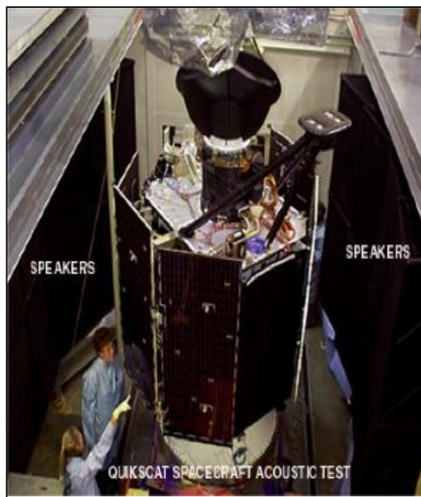
Figure 45—Spacecraft Acoustic Test
