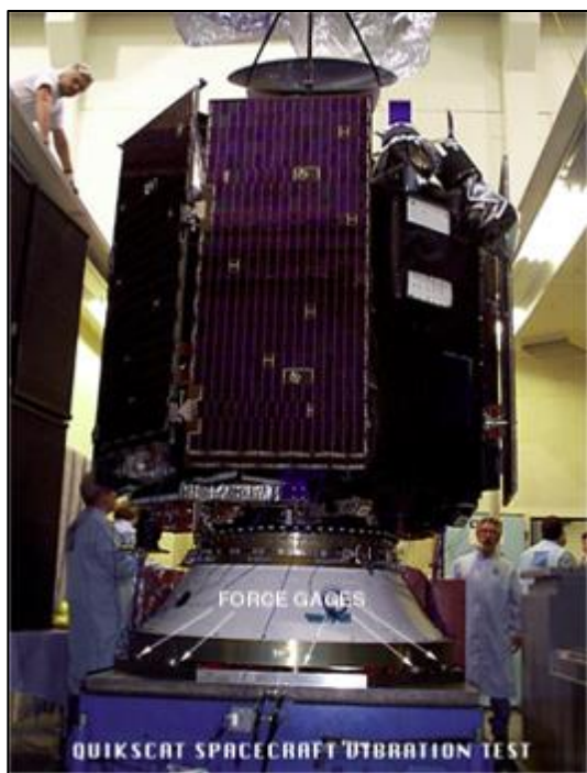
Figure 44—Spacecraft Vibration Test
