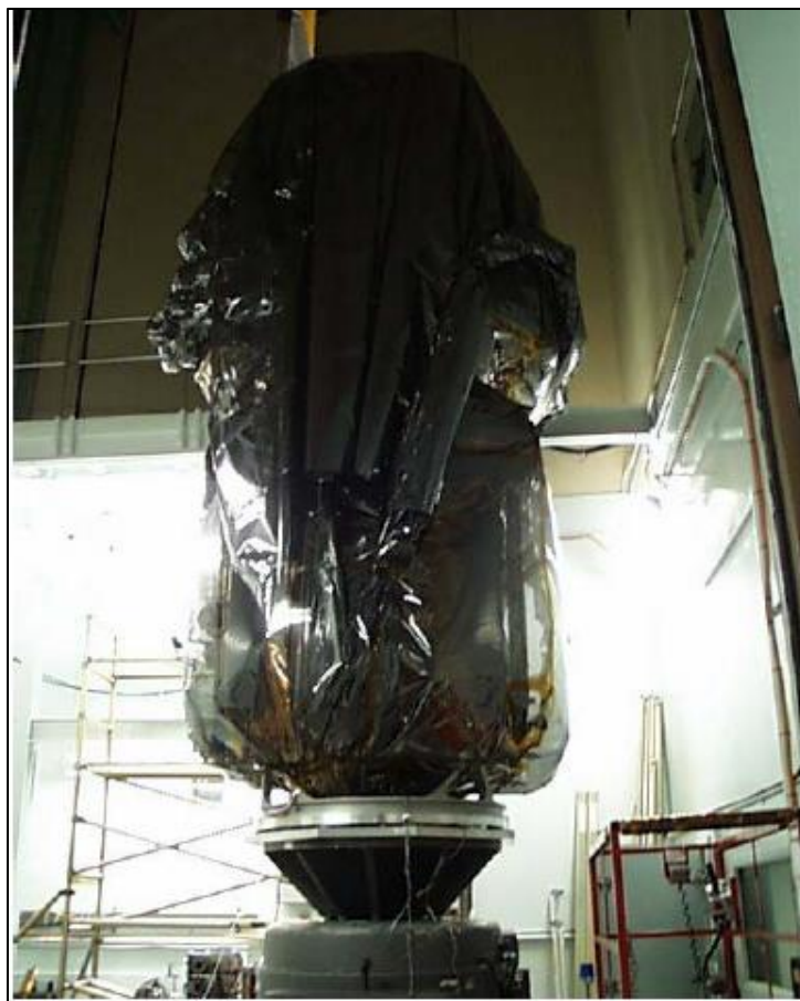
Figure 28—Swift Observatory on Vertical Shaker
