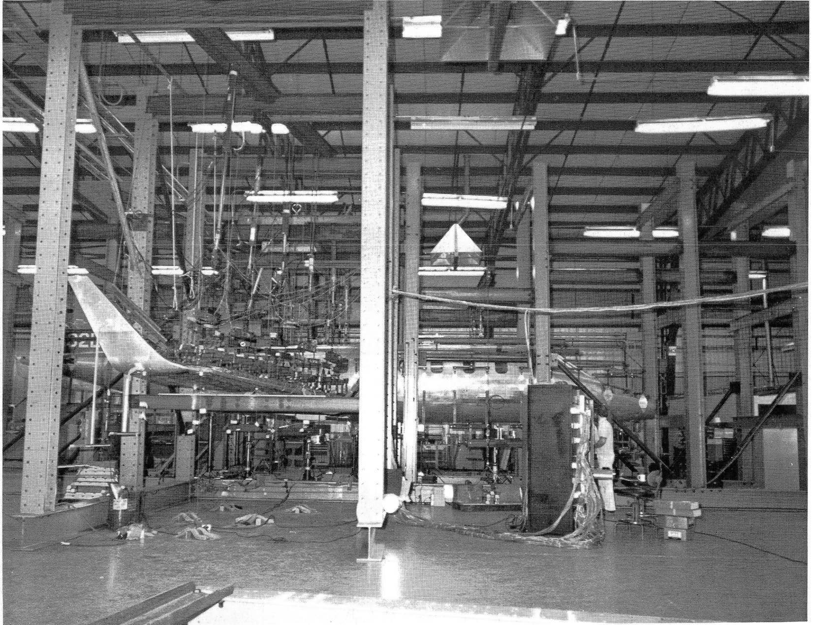
FIGURE 10 - MODEL 28/29 WING STATIC TEST SET-UP
